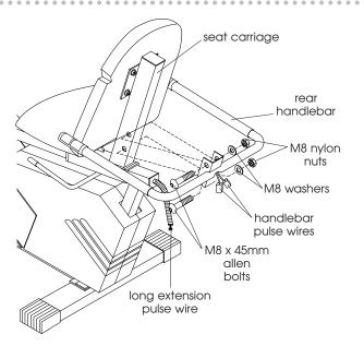
Figure 5 - Install Rear Handlebar
